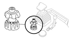
**Figure 15. Trowel Speed Limiter Control**
